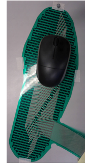
图2 TekScan 压力测量传感器 Fig.2 Transducer of TekScan for pressure measurement
