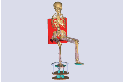
图2 人体与3PH/R踝关节康复机器人耦合模型 Fig.2 Coupling model of human body and 3Ph/R ankle rehabilitation robot
